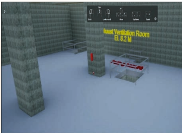
Falling hazards detected prior to the construction of the structure itself through the 3D virtual reality walkthrough.
